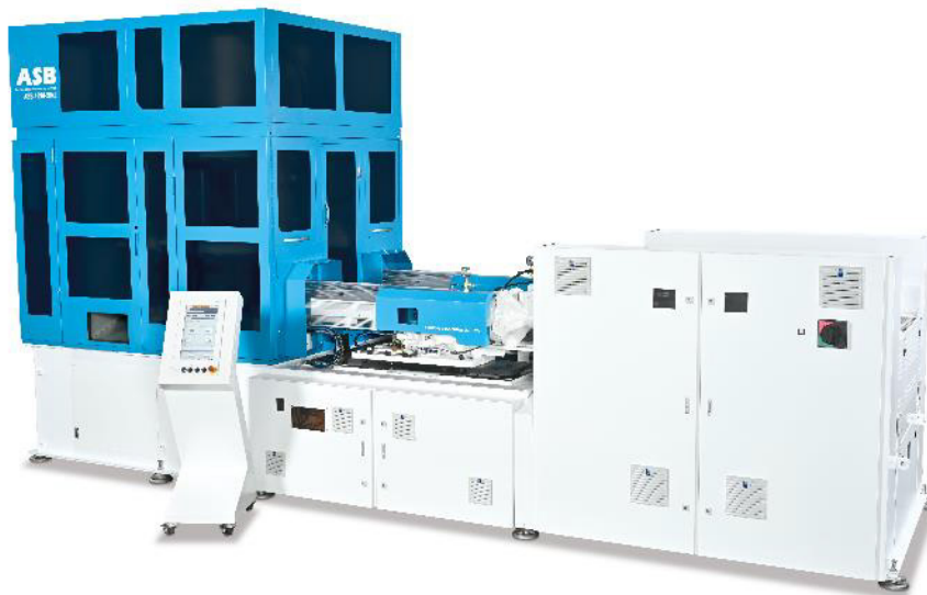
Image 8 - ASB-12M-2INJ Double Layer, One-Step ISBM machine from Nissei ASB
