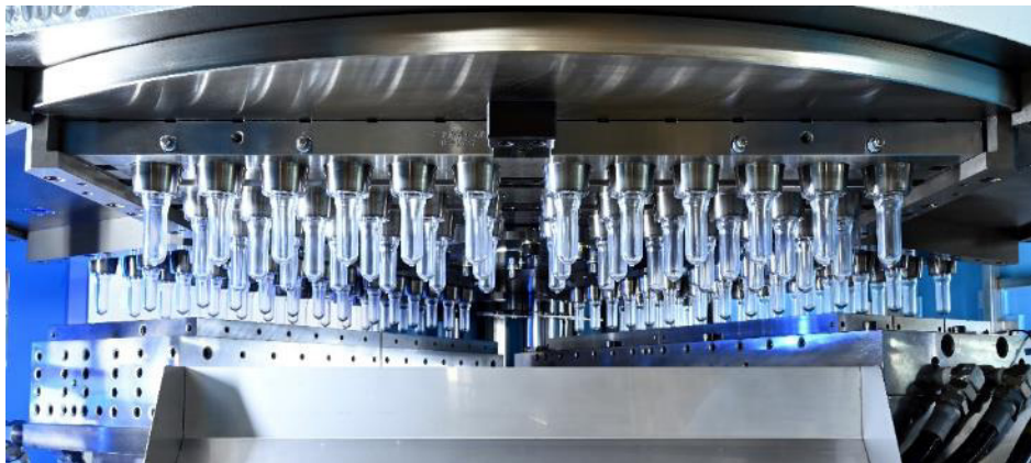
Image 13 - Eject station of PM-100/111N showing rotary table with 36 cavities per station.
