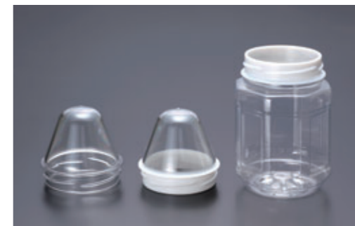
Preform before and after neck crystallization with heat-set PET jar
